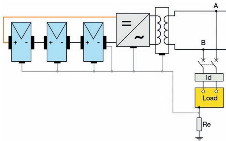
Figure 15 - PV plant with a functionally earthed system
