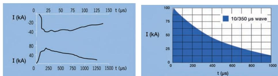
**Figure 19** - Wave shape and intensities of positive (ground to cloud) and negative (cloud to ground) discharges (left). The measured values for intensity of lightning peak current range from hundreds of amperes to several hundred of kiloamperes (right).
