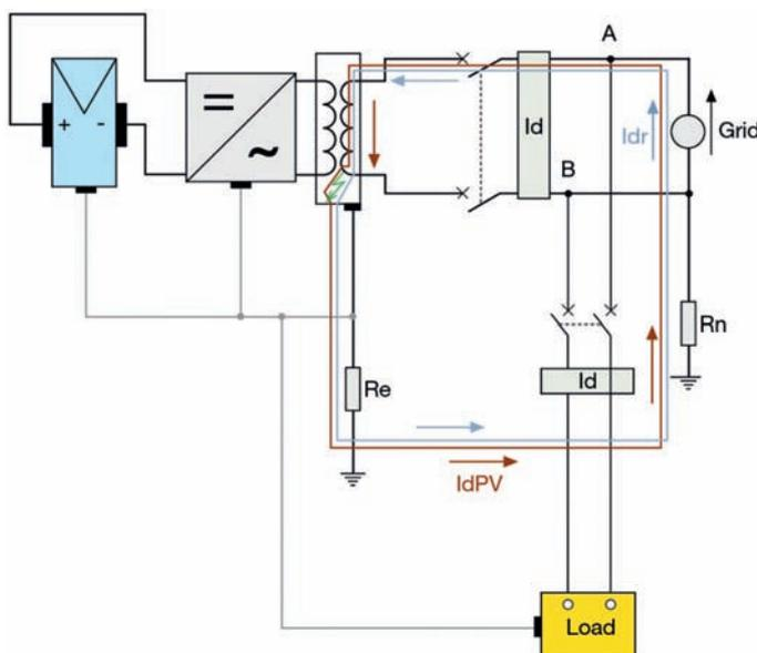
Figure 17 - Current fault example in a floating PV Plant
