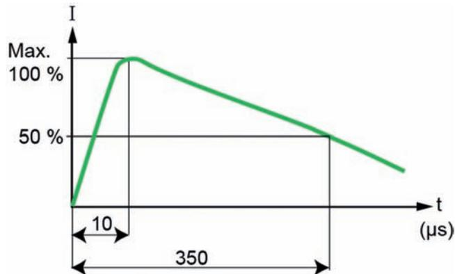
Figure 20 - Direct strike wave model
