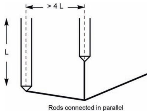
**Figure 5** - Earth rods connected in parallel (Source: Schneider Electric)
