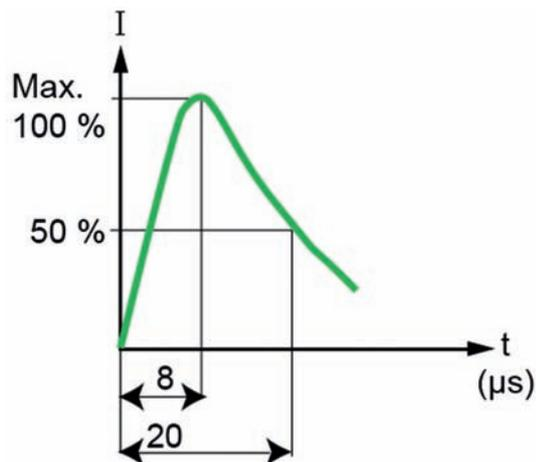
Figure 21 - Indirect strike wave model
