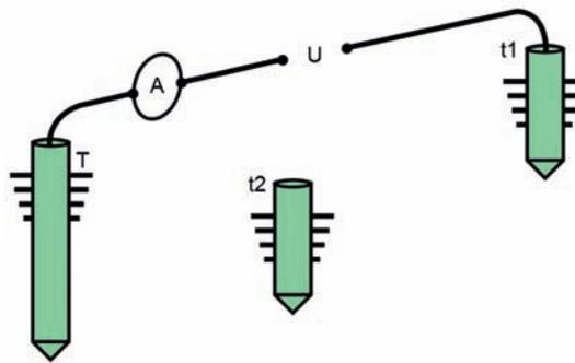
**Figure 7** - Measurement of the resistance to earth of the earth electrode of an installation by means of an ammeter
