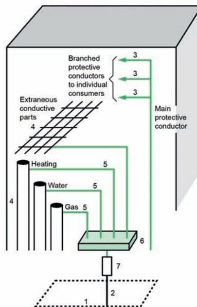
Figure 3 - Components of an earthing system (Source: Schneider Electric)
