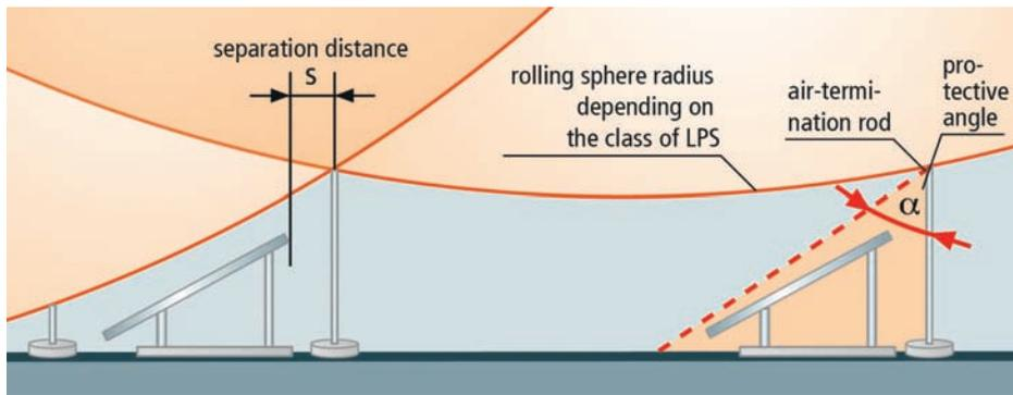
Figure 29 - Rolling sphere method example (Source: Dehn)
