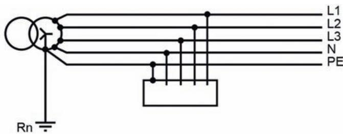
Figure 10 - TN-S System (Source: Schneider Electric)
