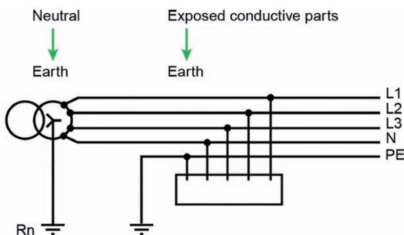
Figure 8 - TT System (Source: Schneider Electric)
