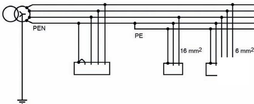
Figure 11 - TN-C-S System (Source: Schneider Electric)
