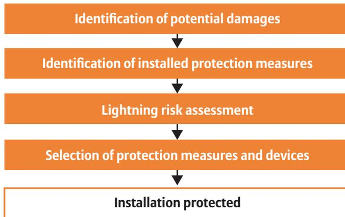
Figure 22 - Steps of the lightning protection assessment process
