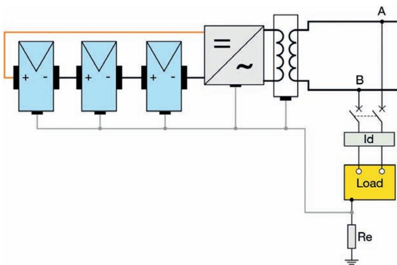
Figure 14 - Plant with isolated PV generator
