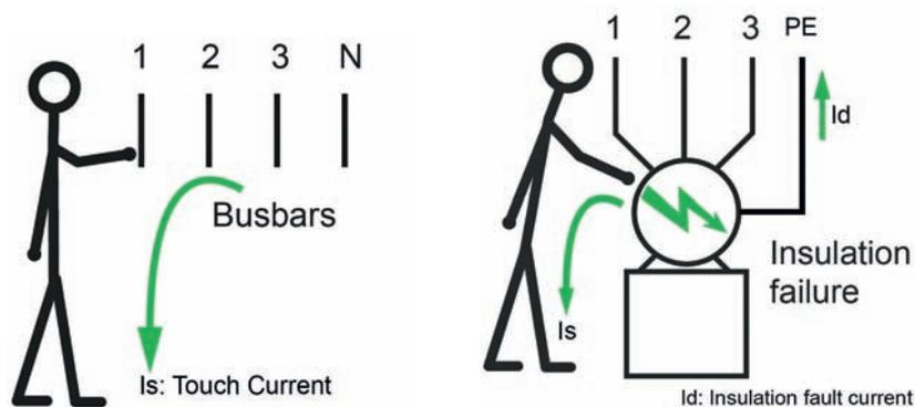
Figure 2 - Direct (left) and indirect (right) contact representations (Source: Schneider Electric)
