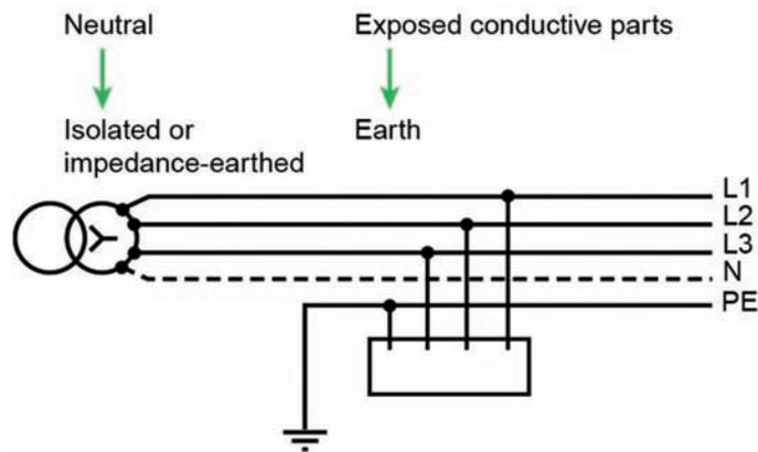
Figure 12 - IT System (Source: Schneider Electric)
