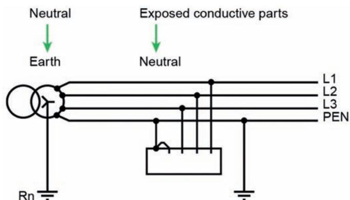
Figure 9 - TN-C System (Source: Schneider Electric)
