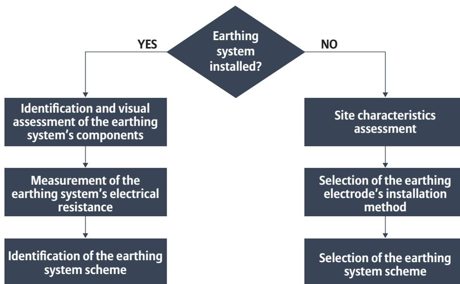
Figure 13 - Steps of the earthing assessment procedure
