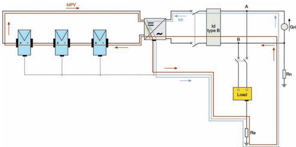
Figure 18 - Current fault example at a plant without galvanic isolation
